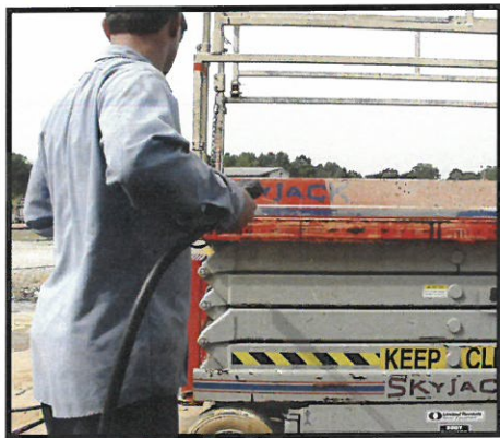
Pressure Wash After Adequate Exposure
