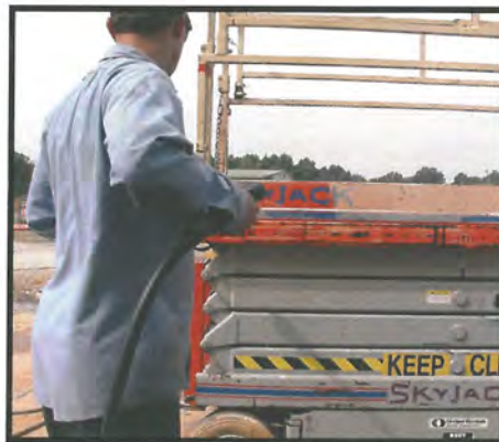
Pressure Wash After Adequate Exposure
