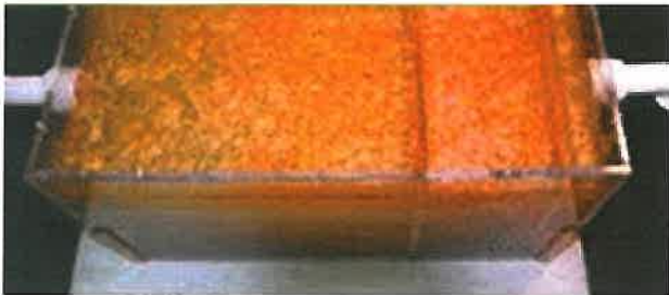
GREASE TRAP SOLIDS BEFORE
