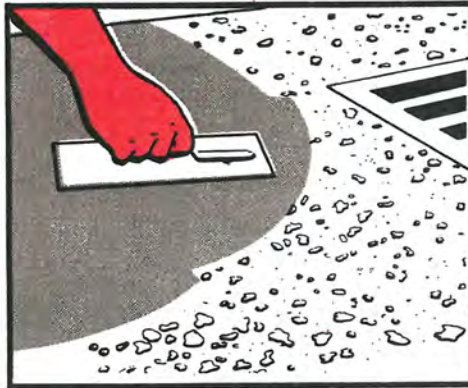
RESURFACES SPALLED OR ERODED SURFACES
