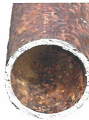
TOWER TREET STOPS corrosion and scale in towers and piping. 1/8 inch of scale thickness causes 10% energy loss!
